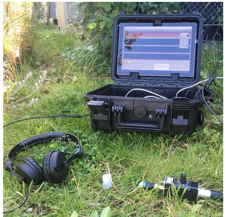
Fig. 6. Mobile recording device with preamplifier and self-built acoustic sensor.
